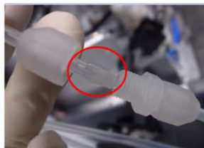
Push carrier gas line into connector.
