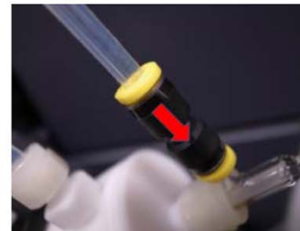
Push connector toward nebulizer (In case of a glass nebulizer).
