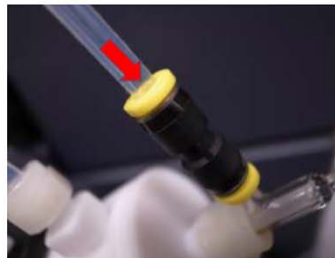
Push carrier gas line into connector (In case of a glass nebulizer).
