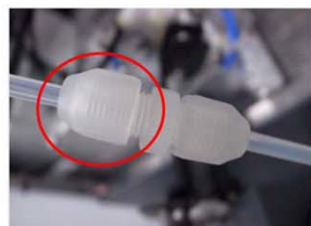
Push carrier gas line into connector (In case of a glass nebulizer).
