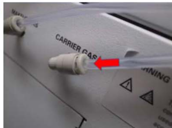
Push carrier gas line into connector.
